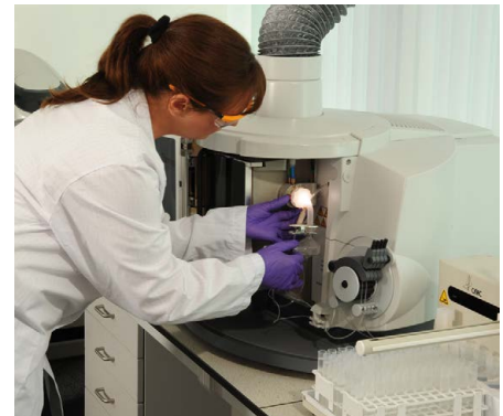
ICP spectrometer of the British company Thermo Scientific fitted with E-T-A type 2210.
