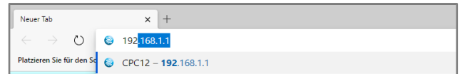
Image 6: Typing the default IP address of the CPC12 webserver in the search field
